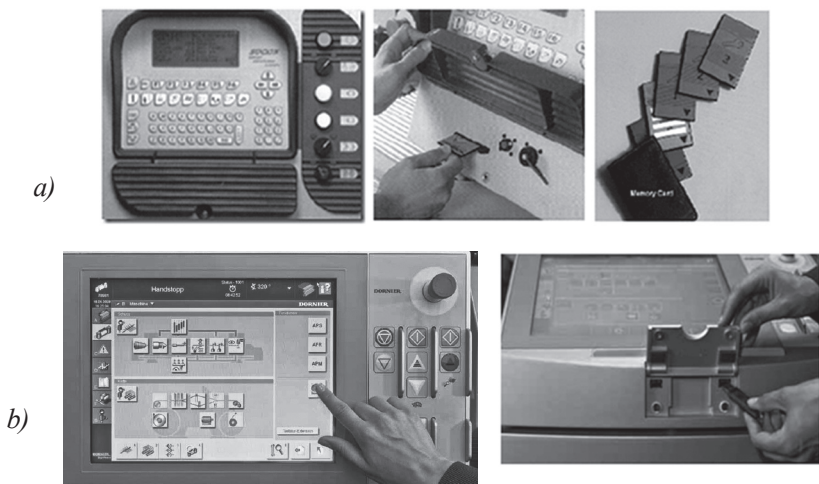
74-rasm. Somet a) va Dornier b) to'quv dastgohlarining elektron nazorat paneli
