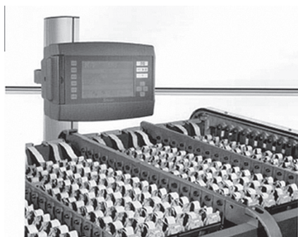
36-rasm. Jakkard mashinasida modullarning joylanishi
