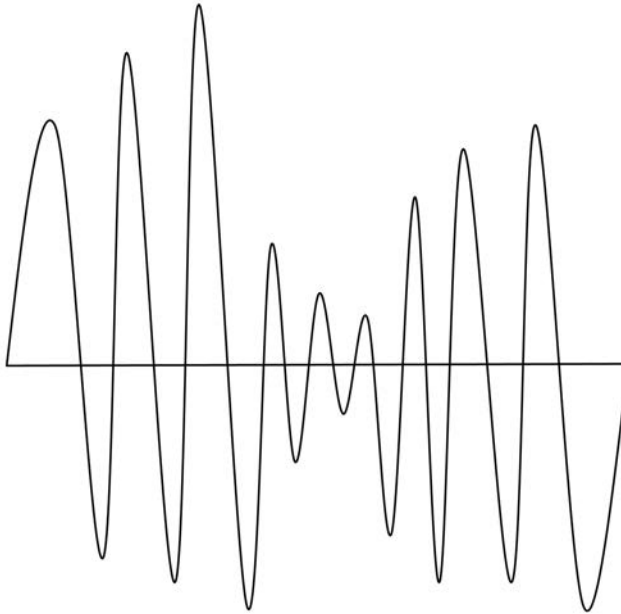
Figure 1.2 With AM, a source modulates the amplitude of a carrier wave.
