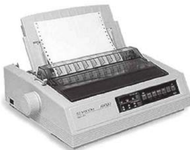
Fig. 1.15. A dot-matrix printer and its character pattern
