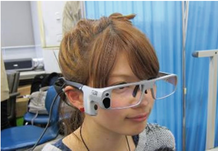
Fig. 6.7 Contact-type eye movement measurement device (Tobii glass eye-tracker manufactured by Tobii). Source Okubo and Takemura (2011)
