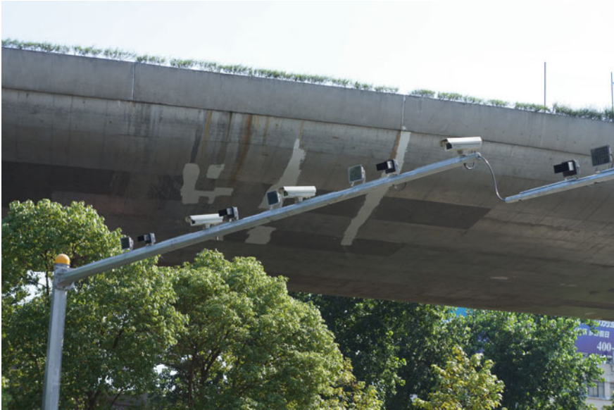
Fig. 1.1 Observer of traffic behavior in breach of institution rules (equipment part): the camera
