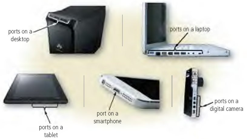
Figure 3-25 Most computers and mobile devices have ports so that you can connect the computer or device to peripherals.
