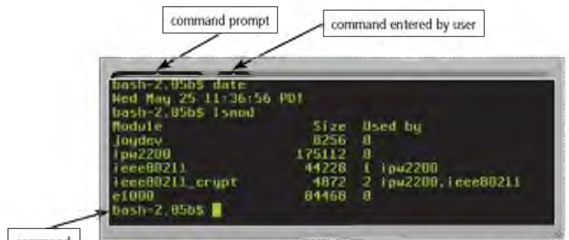
Figure 9-4 A command-line interface requires you to enter exact spelling, form, and punctuation.
