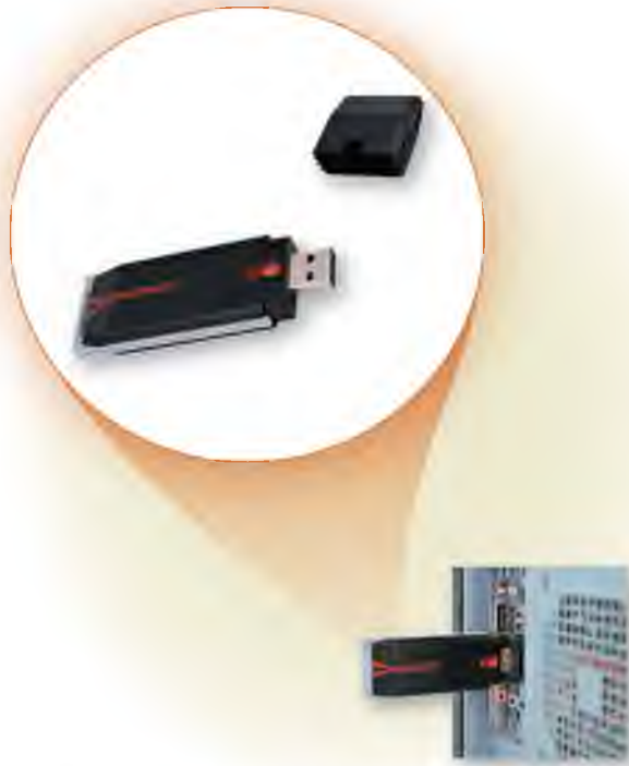
Figure 6-17 A USB adapter inserts into a USB port on a computer or mobile device.
