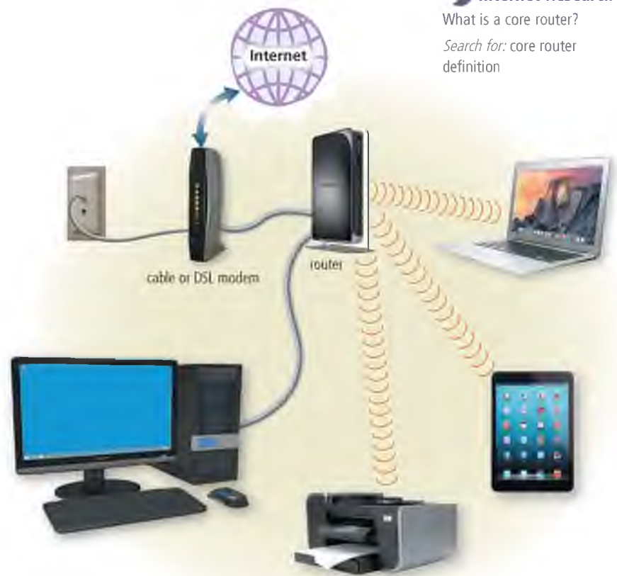
Figure 10-15 Through a router, home and small business networks can share access to a broadband Internet connection, such as through a cable or DSL modem.
