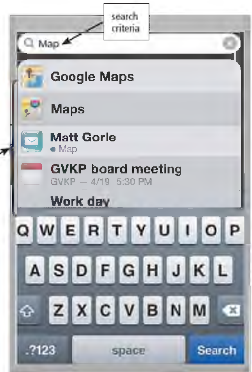
Figure 4-28 This search displays all files on the mobile device that match the search criteria, Map. Notice the search results show map apps, email with a map, and a calendar event. Source: Apple Inc
