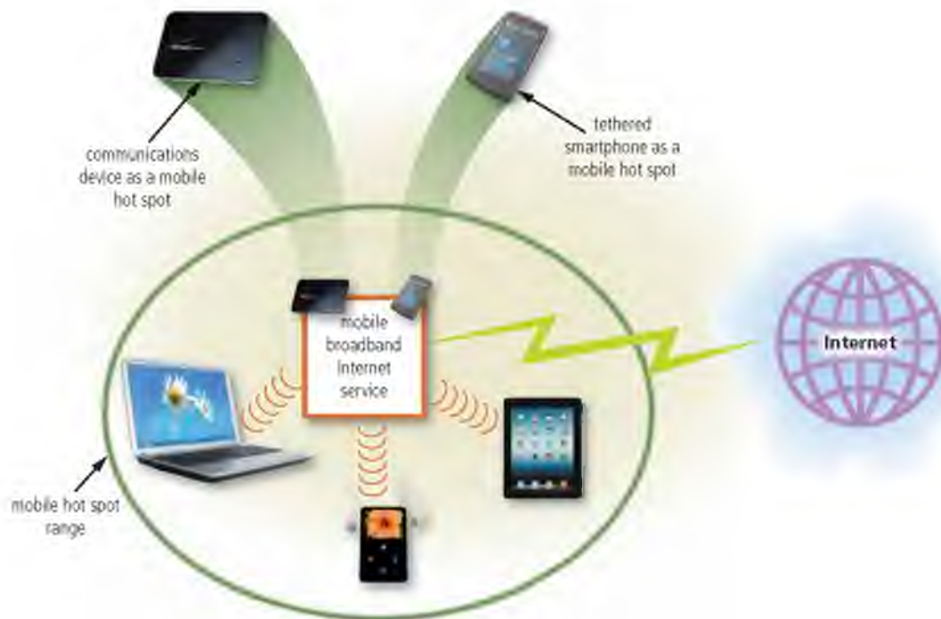
Figure 2-3 You can create a mobile hot spot using a communications device or by tethering a smartphone.
