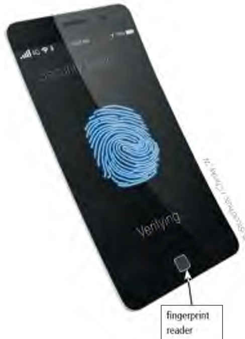
Figure 3-27 Some mobile computers and devices include fingerprint readers, which can be used to verify a user's identity.
