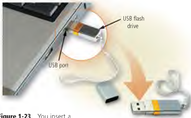
Figure 1-23 You insert a USB flash drive in a USB port on a computer. © Pakhnyushcha / Shutterstock.com
