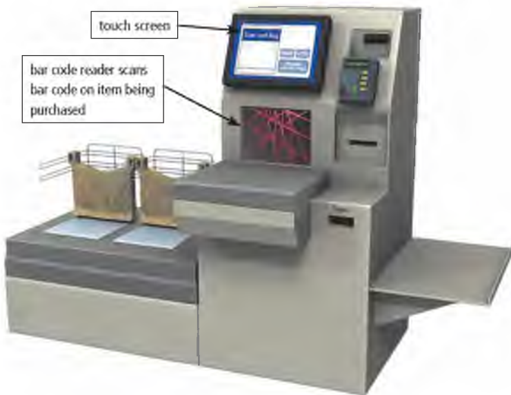
Figure 3-10 Many grocery stores offer self-service checkouts, where consumers use POS terminals to scan purchases, scan their store or saver card and coupons, and then pay for the goods.
