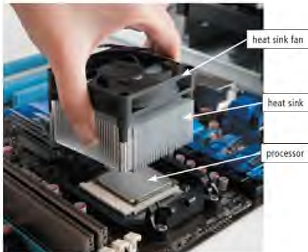
Figure 6-6 This photo shows a heat sink being attached to the top of a processor to prevent the chip from overheating.
