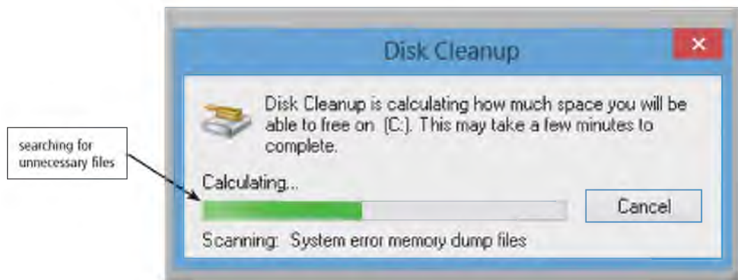
Figure 4-30 A disk cleanup tool searches for and removes unnecessary files.
