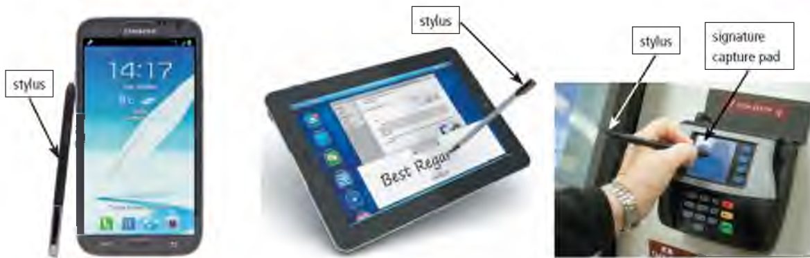
Figure 7-9 You use a stylus to write, draw, or make selections on a touch screen that supports pen input.
