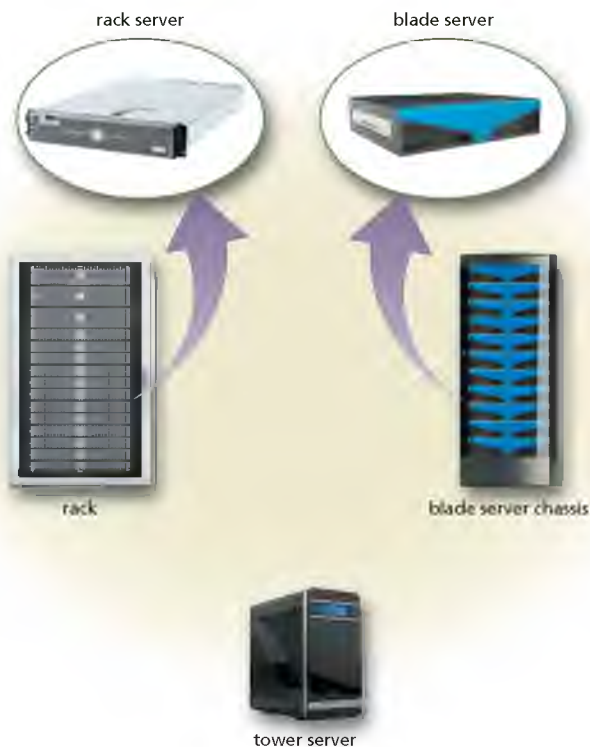
Figure 3-8 Shown here are a rack server, blade server, and tower server.
