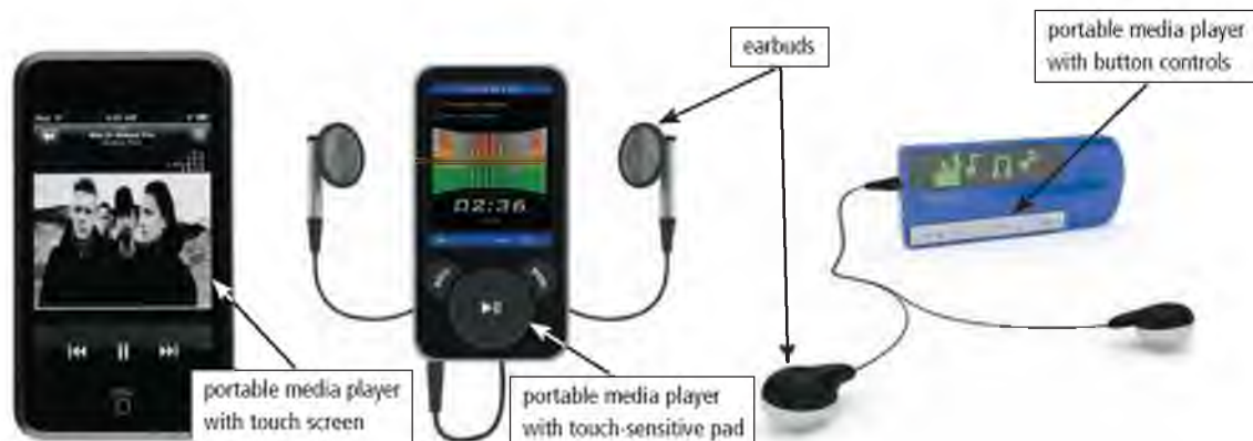
Figure 3-19 Some portable media players have touch screens; others have touch-sensitive pads or buttons that enable you to access your media library.
