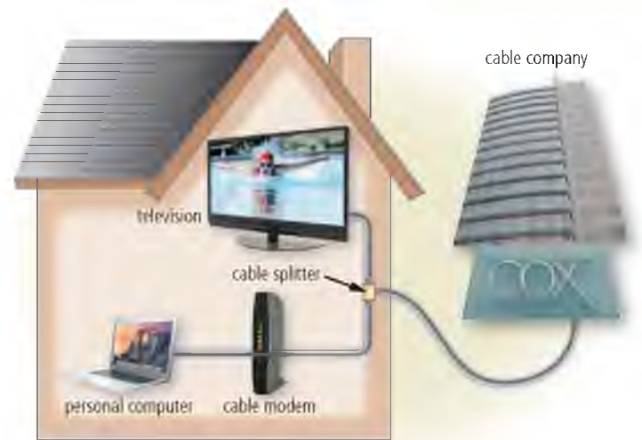
Figure 10-12 A typical cable modem installation.
