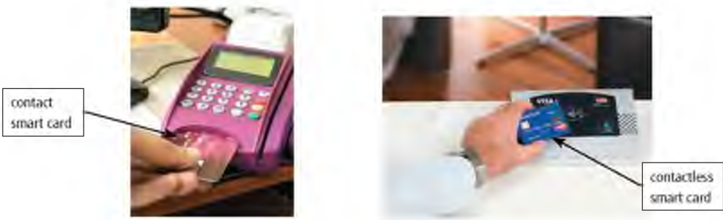
Figure 8-23 Examples of contact and contactless smart cards and their readers. © iStockphoto/oytun karadayi; © iStockphoto/alexander kirch
