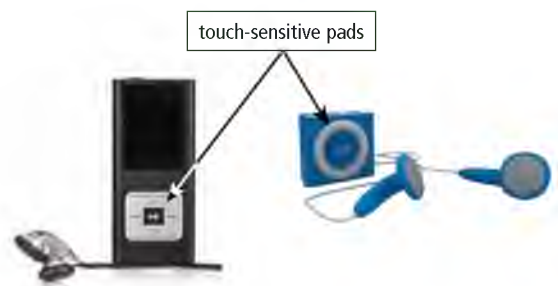
Figure 7-8 You use your thumb or finger to rotate or press buttons on a touch-sensitive pad, which commonly is found on portable media players.
