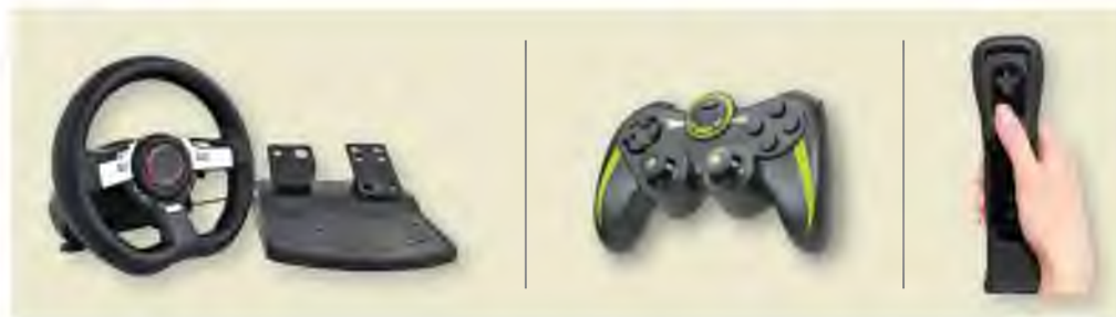
Figure 7-43 Gaming devices often use force feedback, giving the user a realistic experience.
