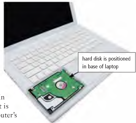
Figure 1-20 A hard disk mounted inside a laptop's case. © iStockphoto / Brian Balster
