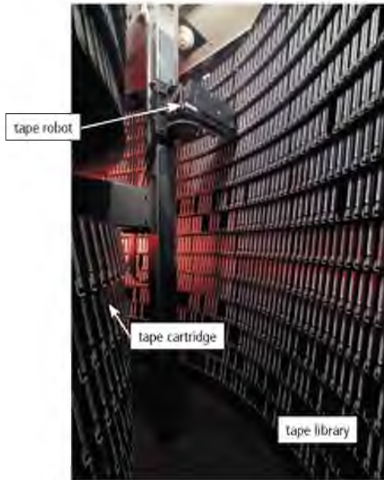
Figure 8-21 A tape robot retrieves tape cartridges.
