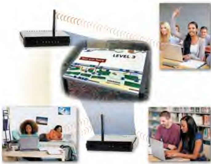
Figure 5-18 Wireless access points or routers around campus allow students to access the school network wirelessly from their classrooms, the library, dorms, and other campus locations.
