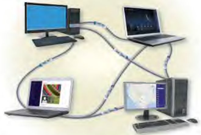
Figure 10-7 As illustrated by the communications in this simplified diagram, each computer or mobile device on a P2P network shares its hardware and software with other computers and mobile devices on the network. Connections can be wired or wireless and may occur through a communications device.
