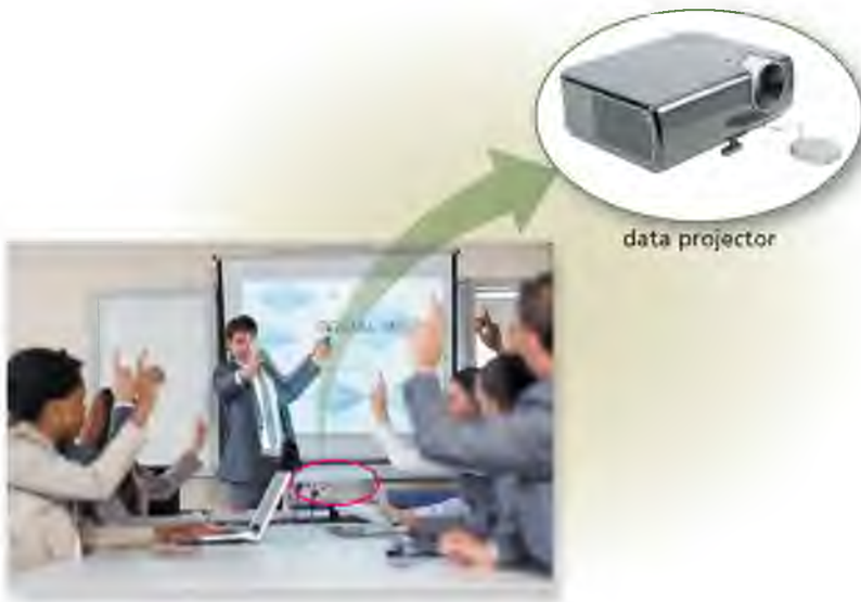
Figure 7-41 A data projector projects an image from a computer or mobile device screen on a larger screen so that an audience easily can see the image.
