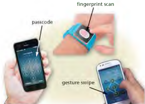
Figure 5-9 Some ways users unlock screens include entering a passcode, scanning a fingerprint, and swiping a gesture.
