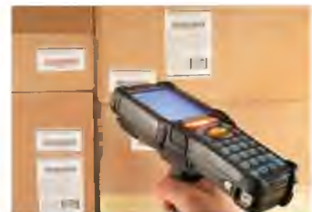
Figure 3-6 This handheld computer is a lightweight computer that enables warehouse employees to take inventory and check supplies.
