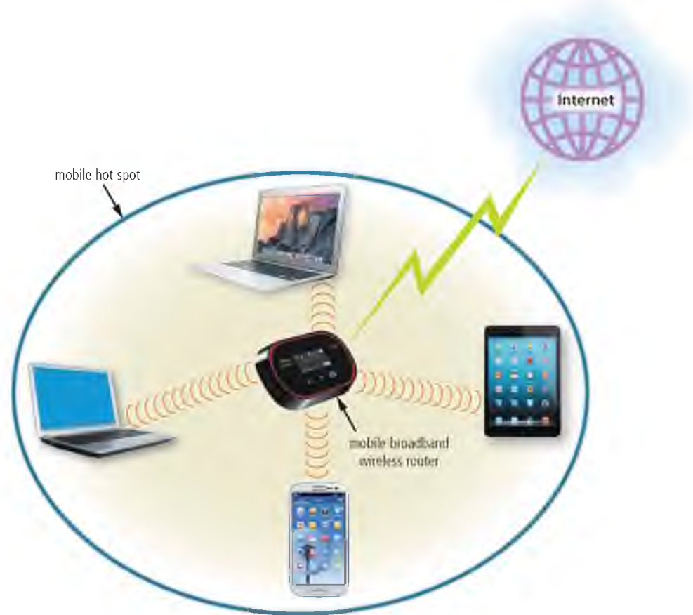
Figure 10-16 Through a mobile broadband wireless router, users can create a mobile hot spot via 3G or 4G mobile broadband Internet service.
