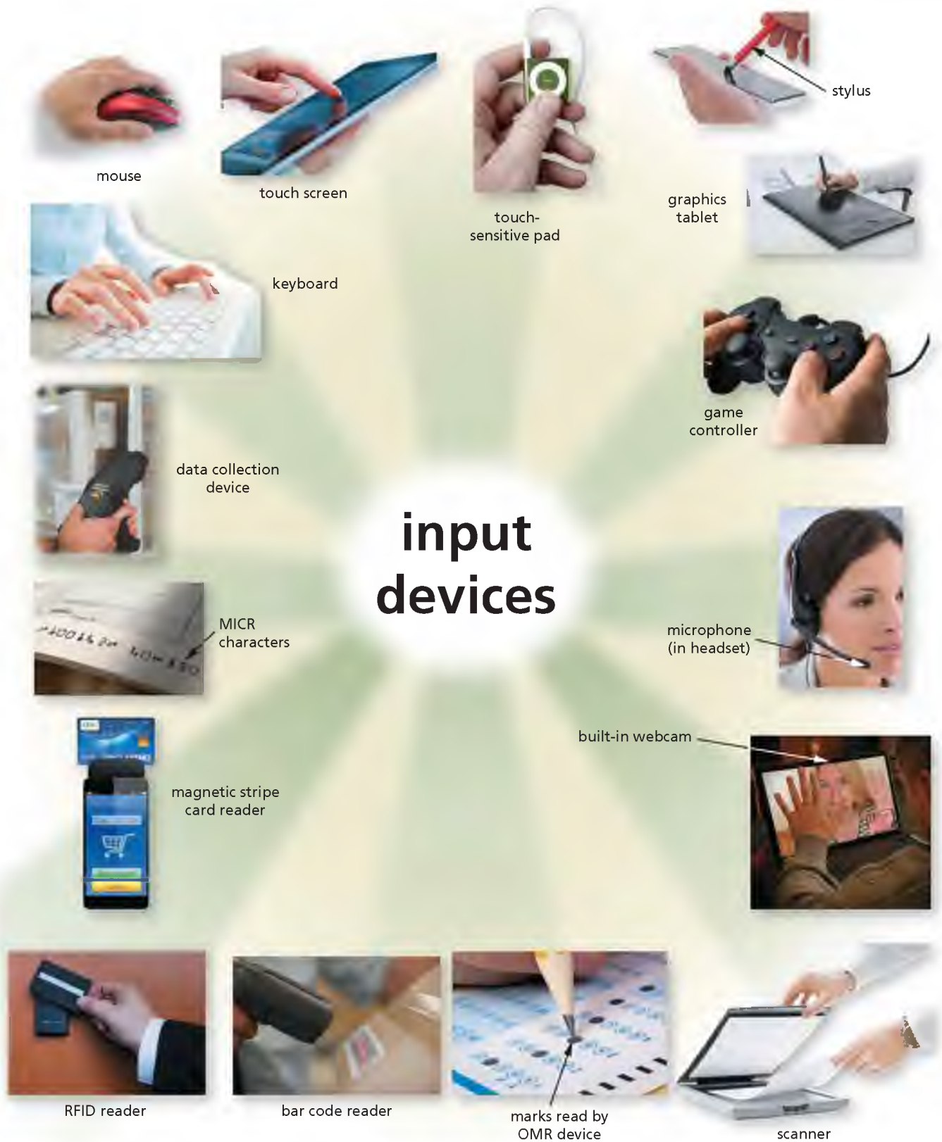
Figure 7-1 Users can enter data and instructions into computers and mobile devices in a variety of ways.
