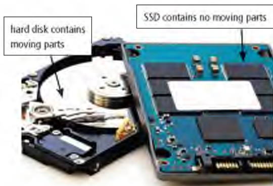
Figure 1-21 A solid-state drive (SSD) is about the same size as a laptop hard disk. © iStockphoto / Ludovit Repko
