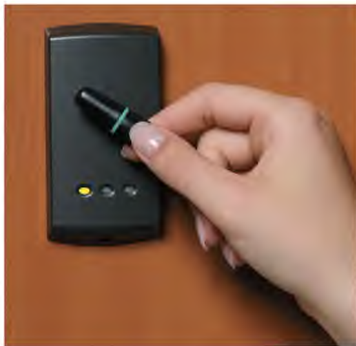
Figure 7-19 This electronic key system locks and unlocks doors using RFID technology.
