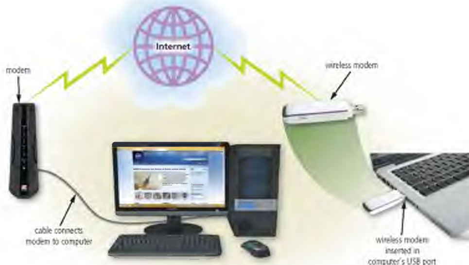
Figure 2-2 Using a modem is one way to connect computers and mobile devices to the Internet.
