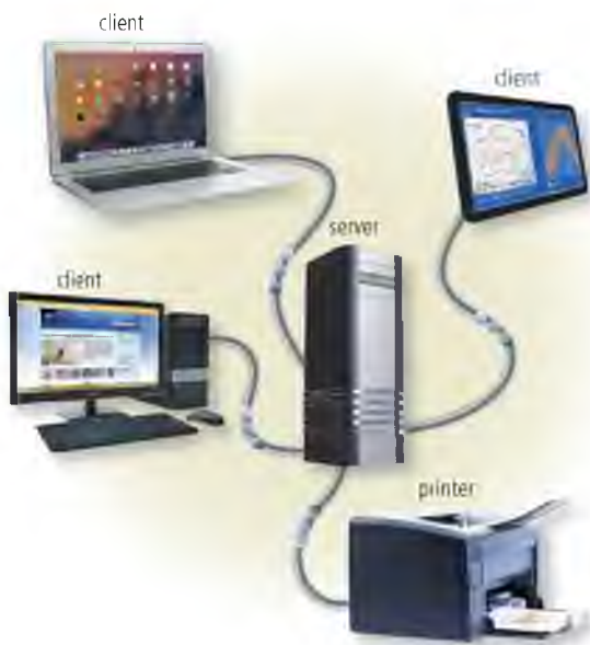
Figure 10-6 As illustrated by the communications in this simplified diagram, on a client/server network, one or more computers act as a server, and the client computers and mobile devices access the server(s). Connections can be wired or wireless and may occur through a communications device.
