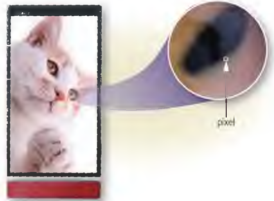
Figure 3-18 A pixel is the smallest element in an electronic image.
