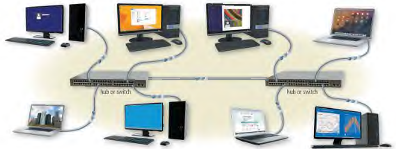
Figure 10-18 A hub or switch is a central point that connects several devices in a network together, as well as connects to other networks, as shown in this simplified diagram.
