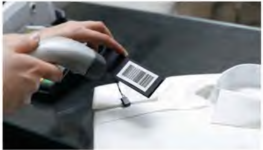
Figure 7-17 A bar code reader uses laser beams to read bar codes on products such as clothing, shown here.
