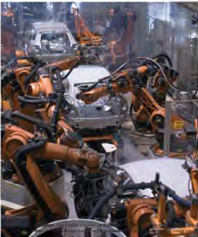
Figure 1-39 Automotive factories use industrial robots to weld car bodies.
