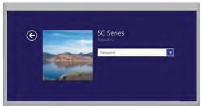
Figure 9-13 Most multiuser operating systems allow each user to sign in, which is the process of entering a user name and a password into the computer. Single-user operating systems often use a password to lock an entire device or computer.
