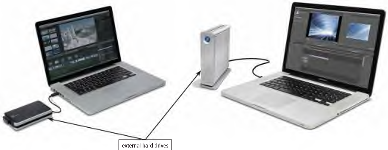
Figure 8-9 Examples of external hard drives. Courtesy of Western Digital; Courtesy of LaCie
