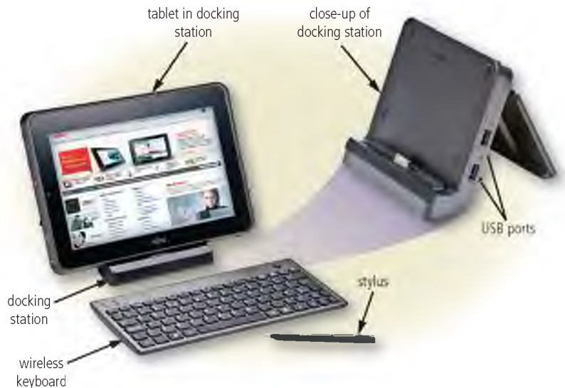
Figure 3-26 Docking stations often are used with tablets and other mobile computers, providing connections to peripheral devices. Courtesy of Fujitsu Technology Solutions; © Cengage Learning
