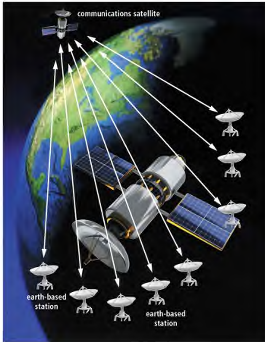
Figure 10-25 Communications satellites are placed about 22,300 miles above the Earth's equator.
