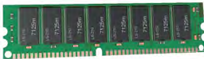
Figure 13 Memory modules contain memory chips.
