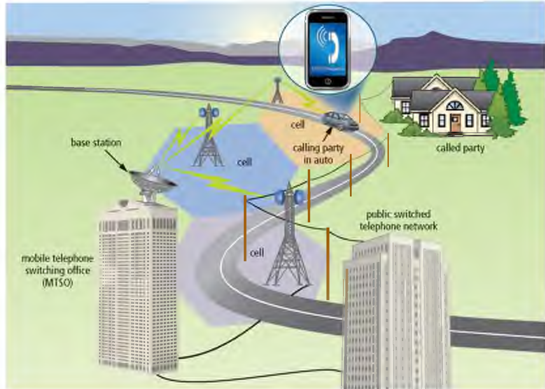
Figure 10-23 As a person with a mobile phone drives from one cell to another, the radio signals transfer from the base station (microwave station) in one cell to a base station in another cell.
