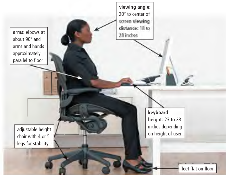
Figure 3-32 A well designed work area should be flexible to allow adjustments to the height and build of different individuals.
