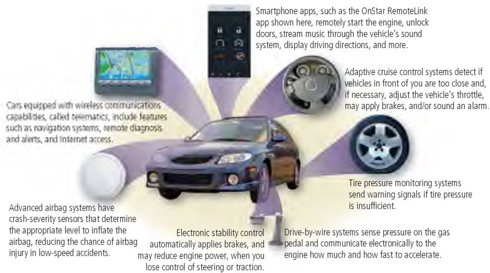
Figure 3-24 Some of the embedded computers designed to improve your safety, security, and performance in today's vehicles.
