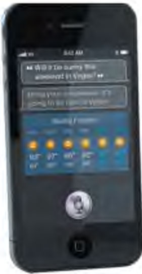
Figure 7-12 With Siri, you can speak instructions and commands to the smartphone and its apps. As shown here, the user asks Siri about the weather, to which Siri replies by speaking a message and displaying the forecast.
