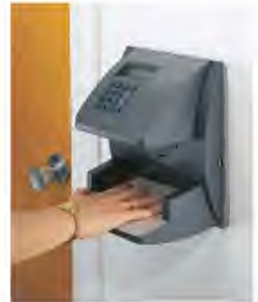
Figure 5-10 A hand geometry system verifies identity based on the shape and size of a person's hand.
