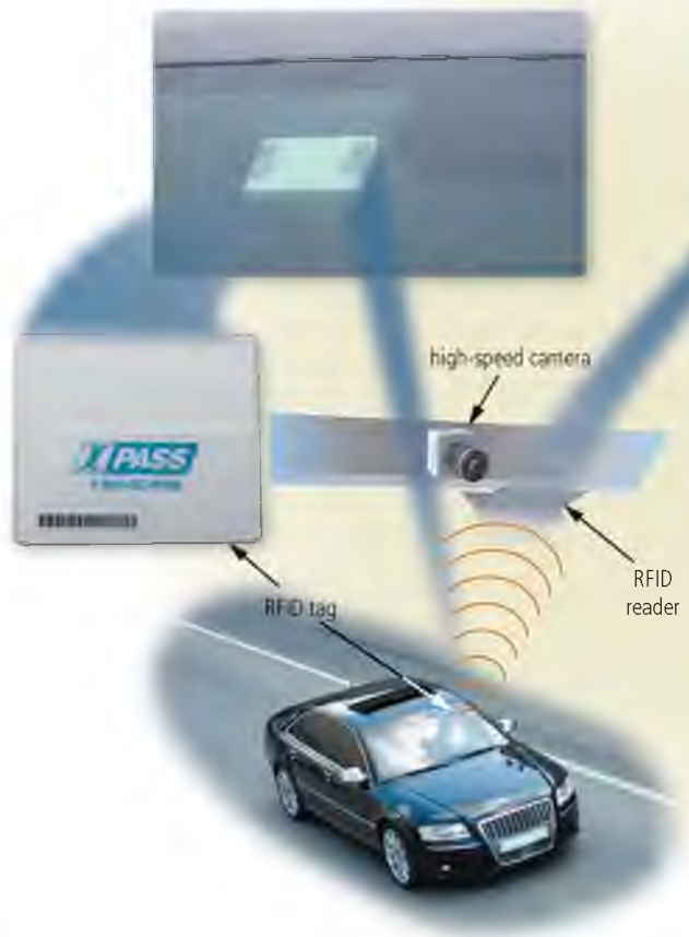
Figure 10-9 This figure shows how electronic RFID toll collection works.
