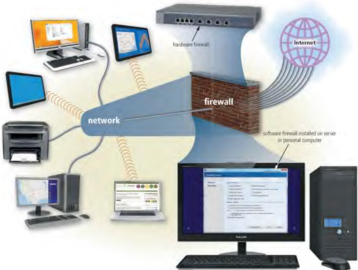
Figure 5-4 A firewall is hardware and/or software that protects a home or business's network resources from intrusion by users on another network, such as the Internet.
