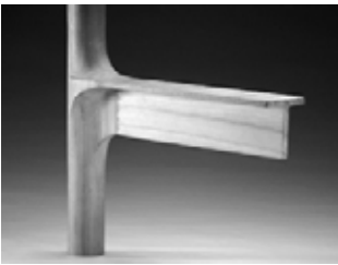
Fig. 10: t-profile joins cylinder perpendicular, final model
