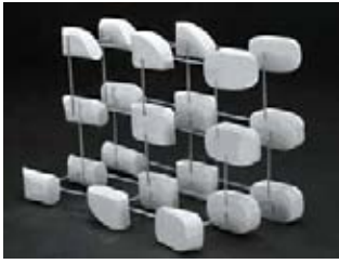
Fig. 13: 3d matrix exploring a continuous circulating fillet in two sizes (small, big); in three different standard orientations (top, side, front); perpendicular interacting with a radius (which starts tangential and ends non tangential), of three varying sizes (zero radius, small radius, big radius).
