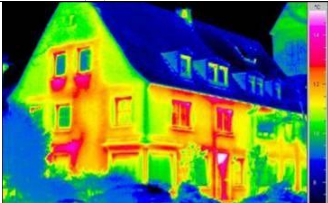
Figure 7.13: Sources of energy losses for a typical commercial building envelope (above), and a thermal image indicating areas of high heat loss (yellow and red areas) from a hotel building
