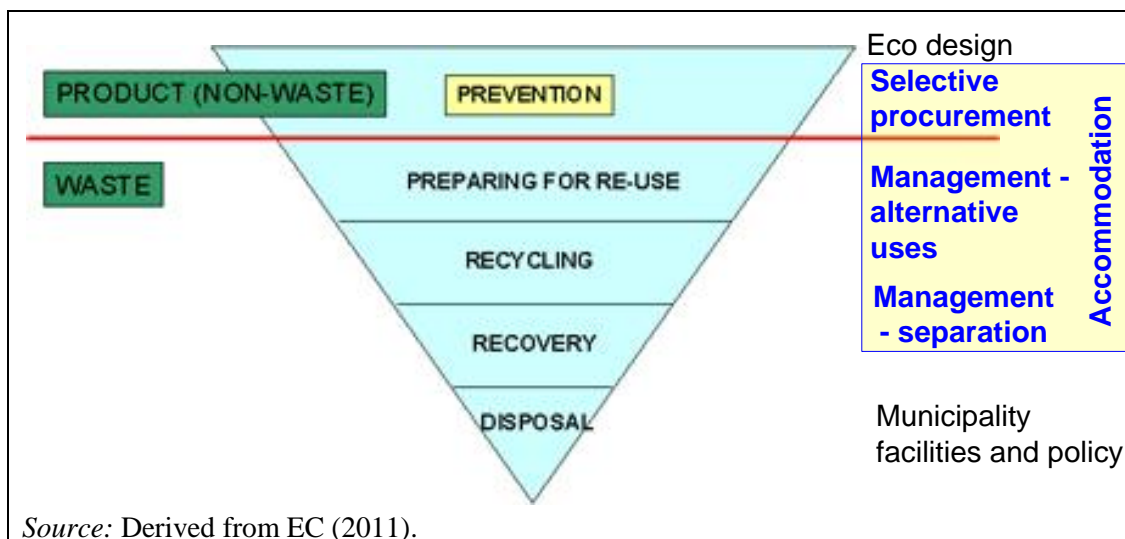
Figure 6.3: The waste management hierarchy, with priority actions at the top
