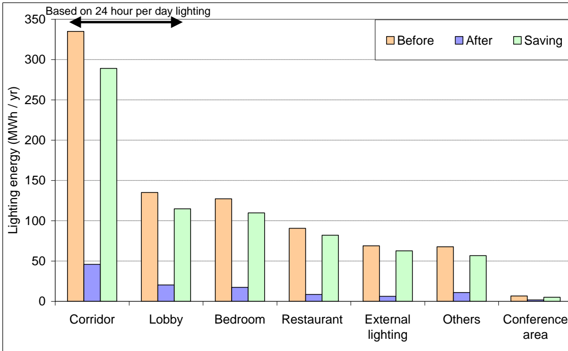
Figure 7.28: Electricity reductions achieved by installation of almost universal LED and CFL lighting in a 65-room hotel, compared with a reference scenario of incandescent, halogen and CFL lighting
